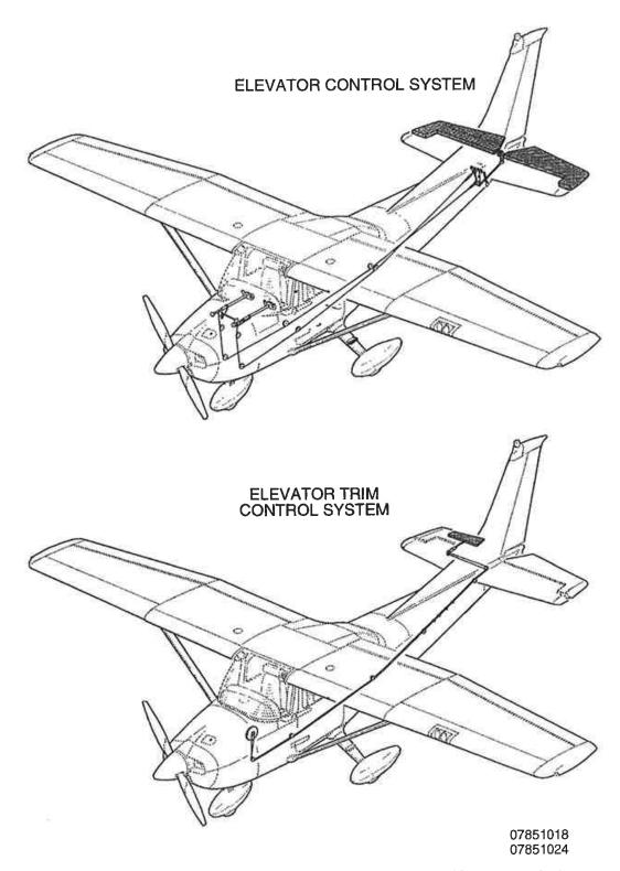
Figure 7-1. Flight Control and Trim Systems (Sheet 2 of 2)
