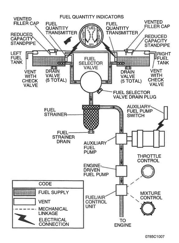
Figure 7-6. Fuel System Schematic
