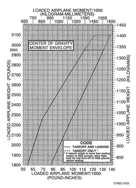
Figure 6-7. Center of Gravity Moment Envelope
