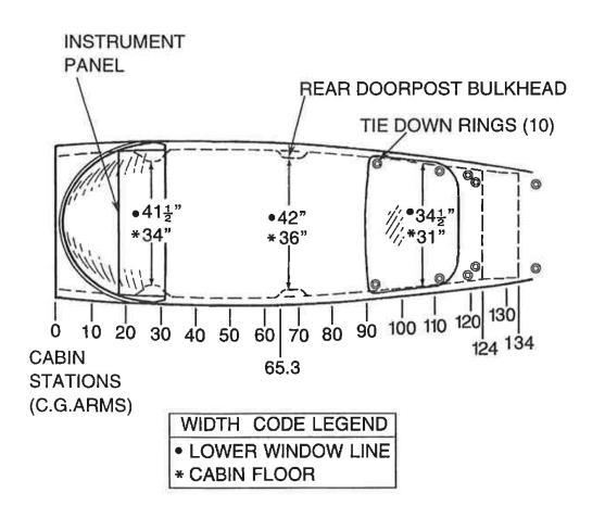
Figure 6-4. Internal Cabin Dimensions (Sheet 2 of 2)
