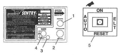
Figure 2. Pointer Model 4000-11 Emergency Locator Transmitter (ELT).
