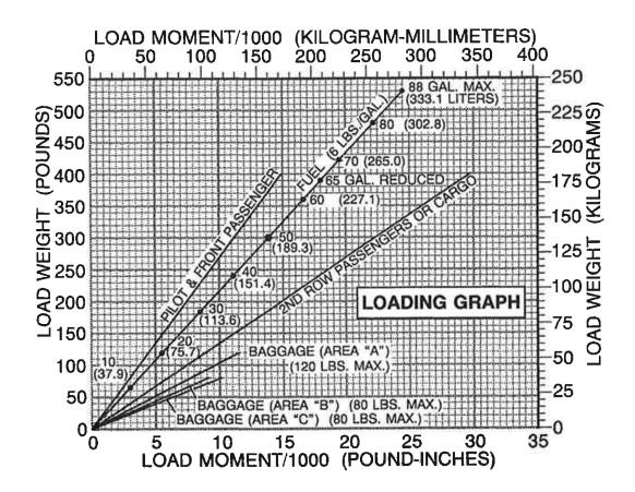
NOTE: Line representing adjustable seats shows pilot and front seat passenger center of gravity on adjustable seats positioned for an average occupant. Refer to the Loading Arrangements diagram for forward and aft limits of occupant C.G. range.
