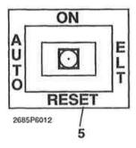
Figure 1. Pointer Model 3000-11 Emergency Locator Transmitter.
