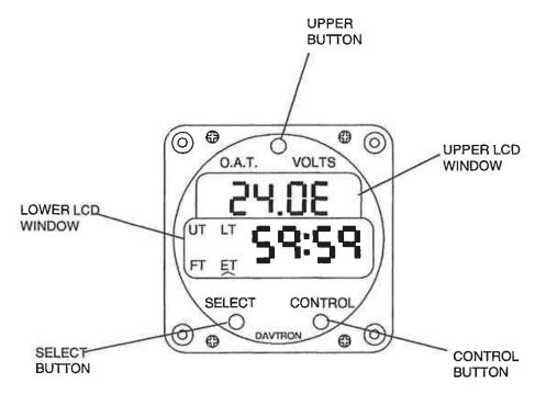
Figure 1. Davtron Model 803 Digital Clock
