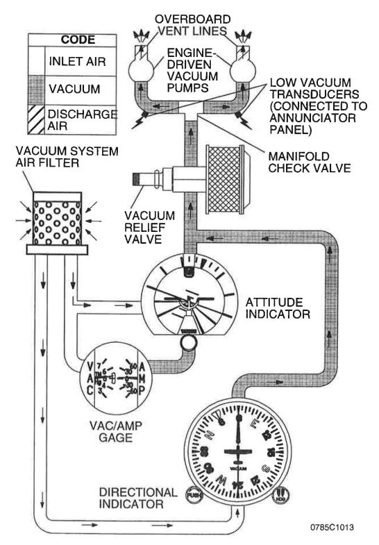
Figure 7-9. Vacuum System Schematic
