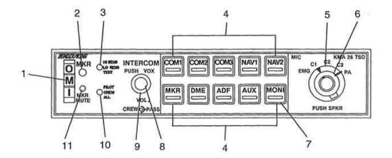
MARKER BEACON ANNUNCIATOR LIGHTS -- The three-light marker beacon receiver built into the KMA 26 gives a visual and aural signal when the ship's antenna passes over a 75 MHz beacon. The blue, amber, and white lights on the faceplate, as well as the audio tones, identify the beacon type.
