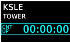
Adds an active timer to the lower right of the display. Use the outer knob to select timer type or select **Start**. Select **Reset** to stop and clear the timer.
