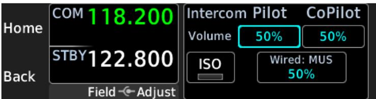
Select control options by turning the outer control knob. The volume control for the pilot's intercom is selected by default. An additional volume control is available for installations wired for intercom music audio.
