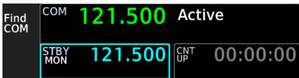
Text within the active window turns cyan to indicate that it is selectable.
