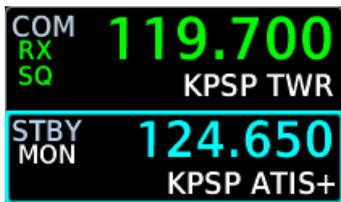
This function automatically displays the facility identifier and frequency type for active and standby frequencies. The unit verifies the displayed frequency against the database at least once per minute.
