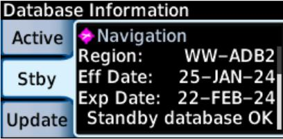
*“Standby database OK” appears at the bottom of the Standby tab whenever a valid database is present on the installed microSD card or in the internal memory.*
