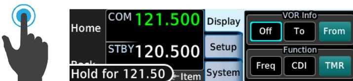
Prior to activation, the "Hold for 121.50" control label appears in the annunciator bar.
