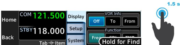
Prior to activation, the "Hold for Find" control label appears in the annunciator bar.
