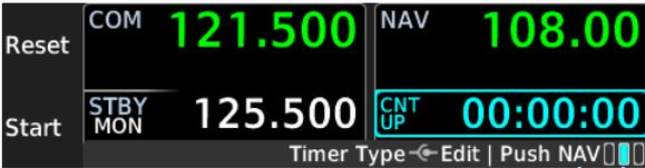
A cyan locator bar indicates active function and knob focus.
