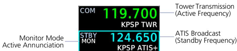
Monitor mode is useful when you want to listen to a recorded broadcast (e.g., ATIS) on the standby channel, but still receive control tower transmissions on the active channel.
