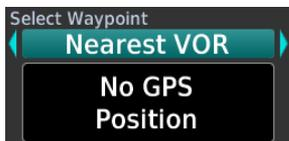
The unit is configured for GPS but is not receiving a position.
