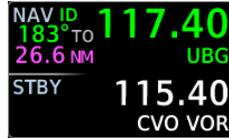
The identifier turns green when a valid ID is decoded from Morse code.
