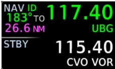
Adds decoded "to" bearing information to the active NAV frequency.
