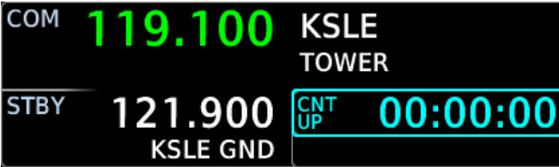
Text shifts beneath the frequency value when you enable right side features.
