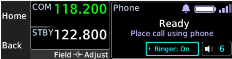
Select control options by turning the outer control knob. The ringer is set to On by default.
