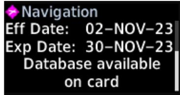
Scroll to the bottom of the tab to see if a standby database is available.
