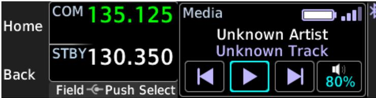
Select control options by turning the outer control knob. An icon at the right of the display indicates when the media player is active.
