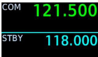
If no action occurs, the STBY window reverts to cyan text after 3 seconds. This indicates that the standby COM frequency is still adjustable using the control knob.
