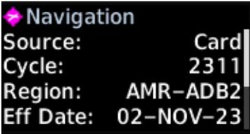
Check the Source field for the current location of the standby database: “Card” or “Internal.”
