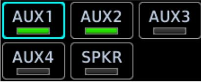
Toggle keys turn a specific function on or off. The current state of the function is indicated below the key label.
