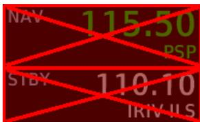
Radio failures are indicated by one or more of the following:
