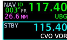
Adds decoded "from" radial information to the active NAV frequency.
