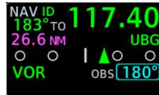
Replaces NAV STBY window with a CDI scale. COM radio is active by default when the frequency is a LOC/LS or a VOR with decoded OBS heading. OBS field is active when manual entry is required.
