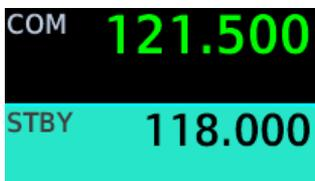
The selected STBY window turns cyan when you use the control knob to change the standby COM frequency.
