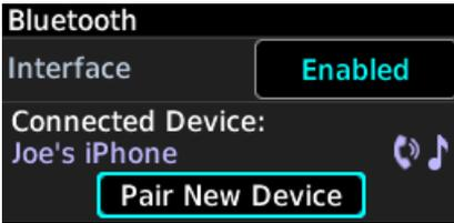
The Bluetooth enabled device name appears upon detection. Depending on the device type, phone and/or media icons appear.
