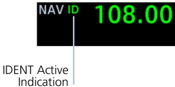
Activate the NAV IDENT function by pushing the **NAV VOL** soft key then the inner control knob.
